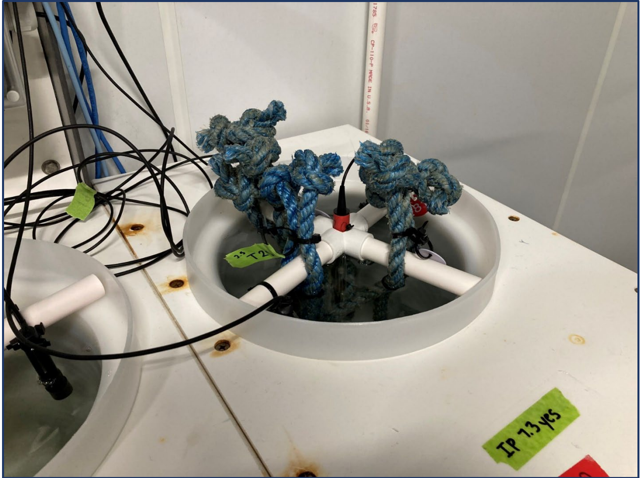
Figure IV.2: Closeup of an experimental aquarium during the Experiment #2 lab trial, featuring the ropes placed once mussels achieved settlement competency (pH probe mounted in the center of the rope rack).
